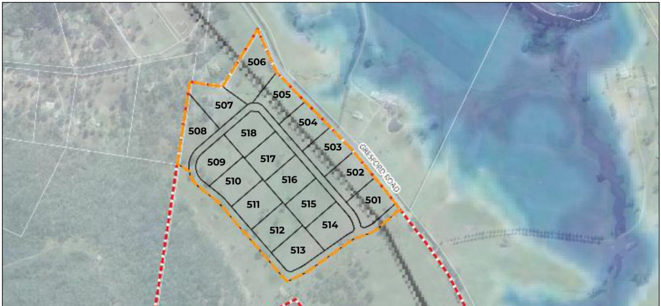
Figure 11: 1% AEP flooding extent (excerpt from IDC (2026))
